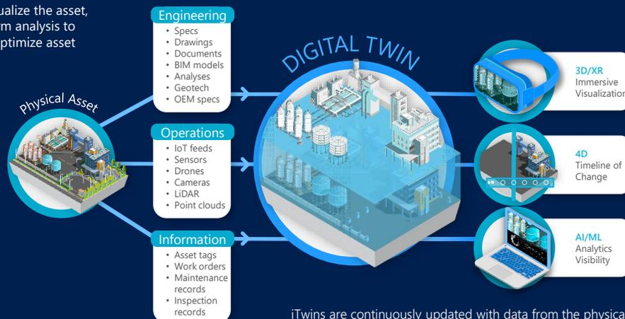
iTwins are continuously updated with data from the physical asset. This data is used to understand and model the asset's performance.
